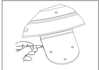
6. Clean roof area where the base feet will be attached to the roof. Do not erase your marks!
